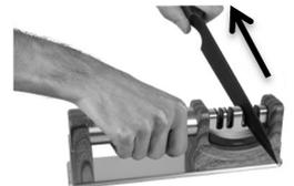
The sharpener has three slots, pull the knife through each slot one by one, from slot 1 to slot 3. Do not sharpen alternately in the three slots.
