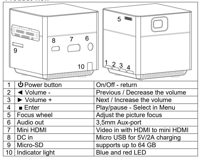
**Power button:** Press this button 5 seconds to shut on or off the device. Short press to return under sub-menu.
