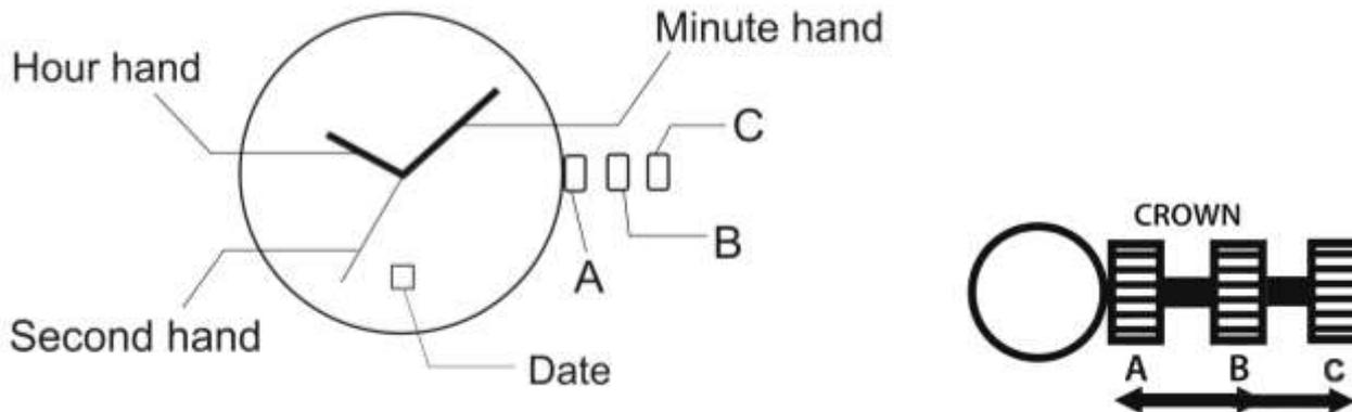
1. Pull the crown out to the "B" position, twist the crown to adjust calendar.
