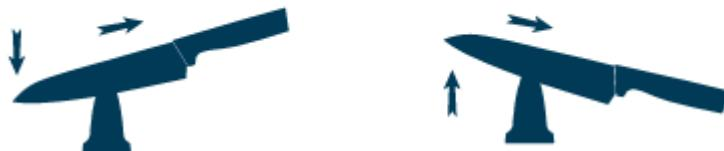
2. For serrated knives, approximately a 30° angle. Keep the blade straight without twisting.
