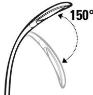
The neck of lamp can be adjusted vertically (up/down) within a 150-degree angle.
