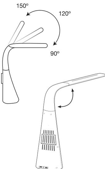
The neck of lamp can be adjusted vertically (up/down) within a 150-degree angle.
