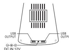
Connect the adaptor into the rear hole of the lamp base and insert the plug in a socket. **Note:** The adapter is exclusively used for this product. It cannot be used on other electric appliances.
