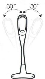
The head of the lamp can be adjusted sideways (right/left) within a 60-degree angle (30 degrees to the left and 30 degrees to the right).
