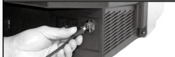
Connect the end of the coaxial cable to the RF input socket of TV set.
