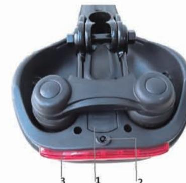
1. Battery Compartment (1x3V CR2032 battery is included )
