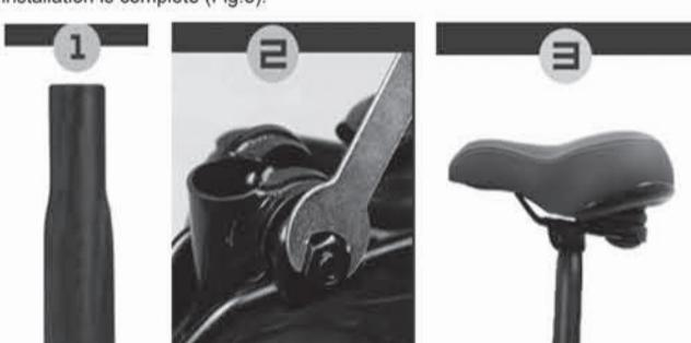
**Option 2** (Bike saddle post like Fig. A): Remove the nuts on both sides of the new saddle with a wrench (Fig.B), draw out the crossbar and other parts (Fig.C). Assemble the new saddle on the saddle post , adjust the saddle titling angle and tighten the original screw of the saddle post (Fig.E). The installation is complete (Fig.F).
