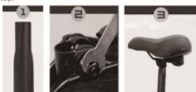
**Option 2** (Bike saddle post like Fig. A): Remove the nuts on both sides of the new saddle with a wrench (Fig.B), draw out the crossbar and other parts (Fig.C). Assemble the new saddle on the saddle post ,adjust the saddle titling angle and tighten the original screw of the saddle post (Fig.E). The installation is complete (Fig.F).
